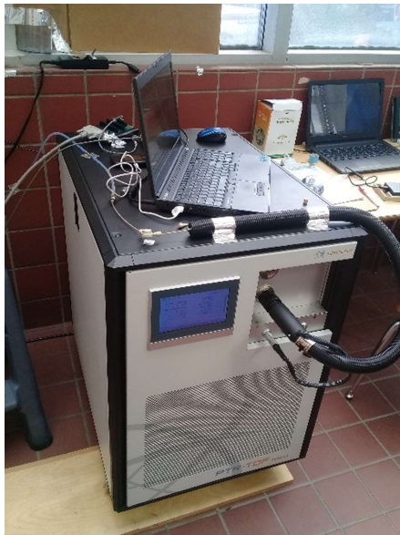
Figure 4c. Volatile organic compound monitoring systems. The PTR-TOF-MS (picture on the left) and sampler and sorbent tubes for GC-MS (picture on the right) in the greenhouse at Harriet Tubman Middle School.
