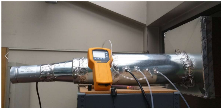
Figure 2. Left: Installation of steel inlet duct in indoor location inside HTMS. The leftmost component of the inlet duct is a continuously operating ventilation fan that maintained a high refresh rate inside the duct. Right: Approximate location of sampling inlet on HTMS building. Note that all air quality sampling conducted here is that of outdoor air; Phase II of the project will include indoor air monitoring.
