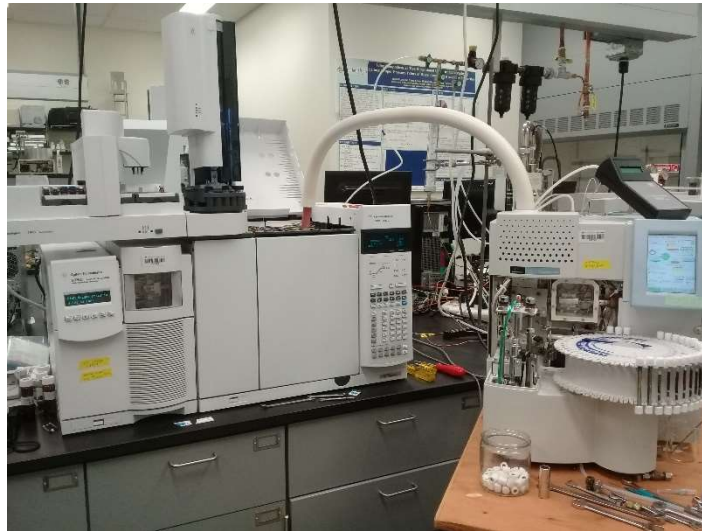
Figure 4d. TD-GC-MS in the lab at PSU for the analysis of sorbent tubes
