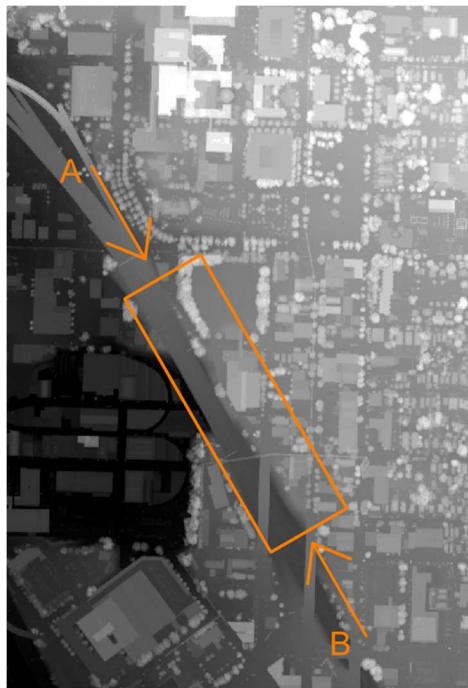
Figure 28. Elevation map of the site and surrounding area. Arrow A shows the wind direction for April through September while arrow B shows the wind speed for October through March. The rectangle centered about the school indicates the region of interest for the scale model.
