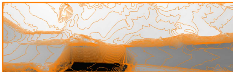
Figure 30. Elevation contours each line represents a 0.5 m elevation change. Topography model is made of layers per the contours.
