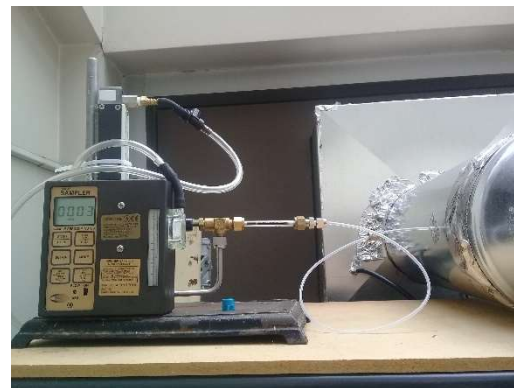
Figure 4c. Volatile organic compound monitoring systems. The PTR-TOF-MS (picture on the left) and sampler and sorbent tubes for GC-MS (picture on the right) in the greenhouse at Harriet Tubman Middle School.
