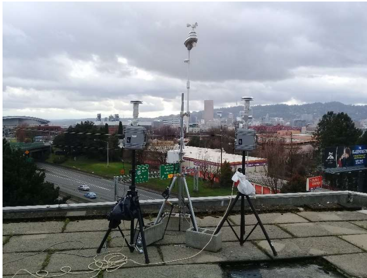
Figure 4b. Weather station between the two ARA samplers at Harriet Tubman Middle School (picture on the left) and an ARA sampler (PM10) (picture on the right)
